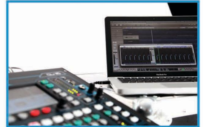
The returns from the Mac can be assigned to the Input channels. The interface is class-compliant on Mac OS X – which means it's truly plug 'n play, with no need to install a driver. It will be recognized straightaway by any DAW supporting Core Audio, including Logic, Cubase, Reaper, and Pro Tools.
